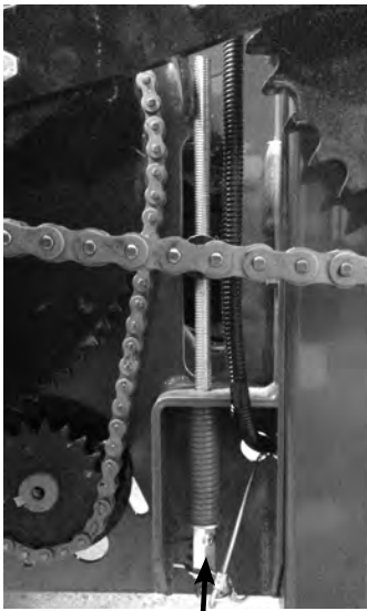
Left Side Apron Tightener Bolt
