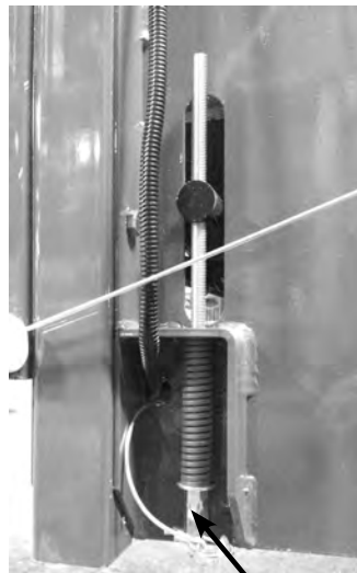
Right Side Apron Tightener Bolt
